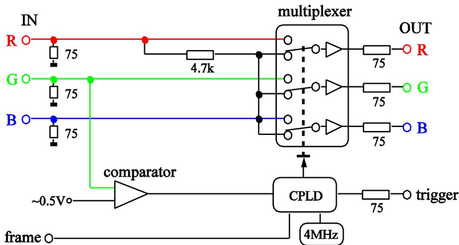
Fig 1. The schematic of a video switcher. The multiplexer has two groups of input, controlled by a voltage level. When it is in the mode shown above, the RGB channels of a monitor receive the same signal, so the display is in grayscale. The switching voltage is generated by a CPLD chip, controlled by green signal. The trigger is also controlled by green signal. Circuit may change without notice.
